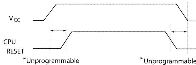
$\overline{RES}$  should be kept at  $V_{SS}$  level when  $V_{CC}$  is turned on or off. The EEPROM breaks off programming operation when  $\overline{RES}$  becomes low, programming operation doesn't finish correctly in case that  $\overline{RES}$  falls low during programming operation.  $\overline{RES}$  should be kept high for 10 ms after the last data input.
