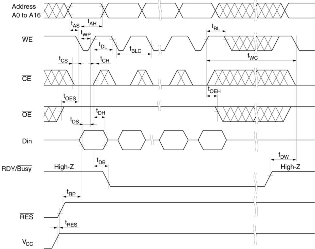
FIGURE 5. PAGE WRITE TIMING WAVEFORM(2) ( $\overline{CE}$  CONTROLLED)
