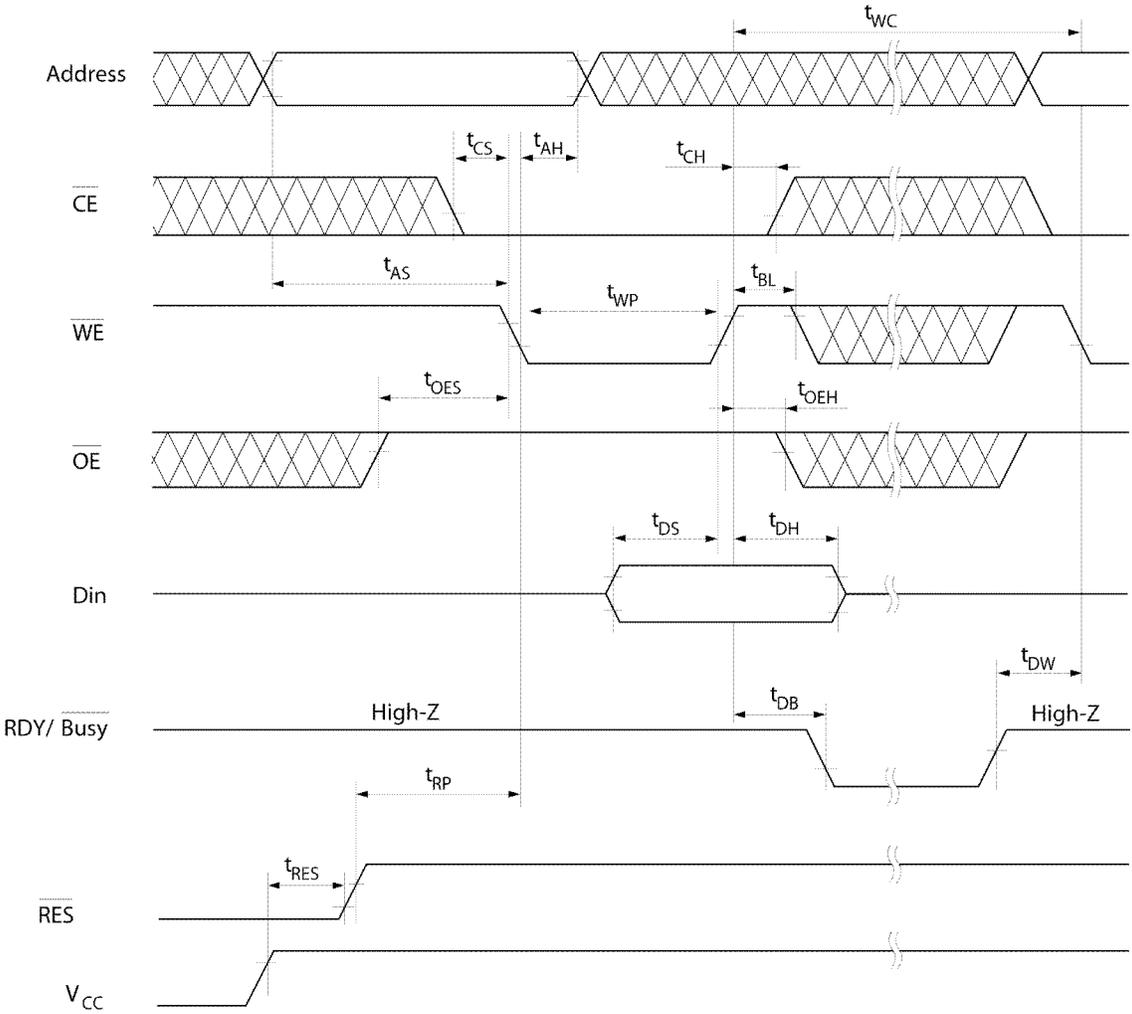
FIGURE 3. BYTE WRITE TIMING WAVEFORM (2) ( $\overline{CE}$  CONTROLLED)
