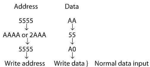
Software data protection mode can be canceled by inputting the following 6 bytes. Then, the EEPROM turns to the non-protection mode and can write data normally. However, when the data is input in the canceling cycle, the data cannot be written.
