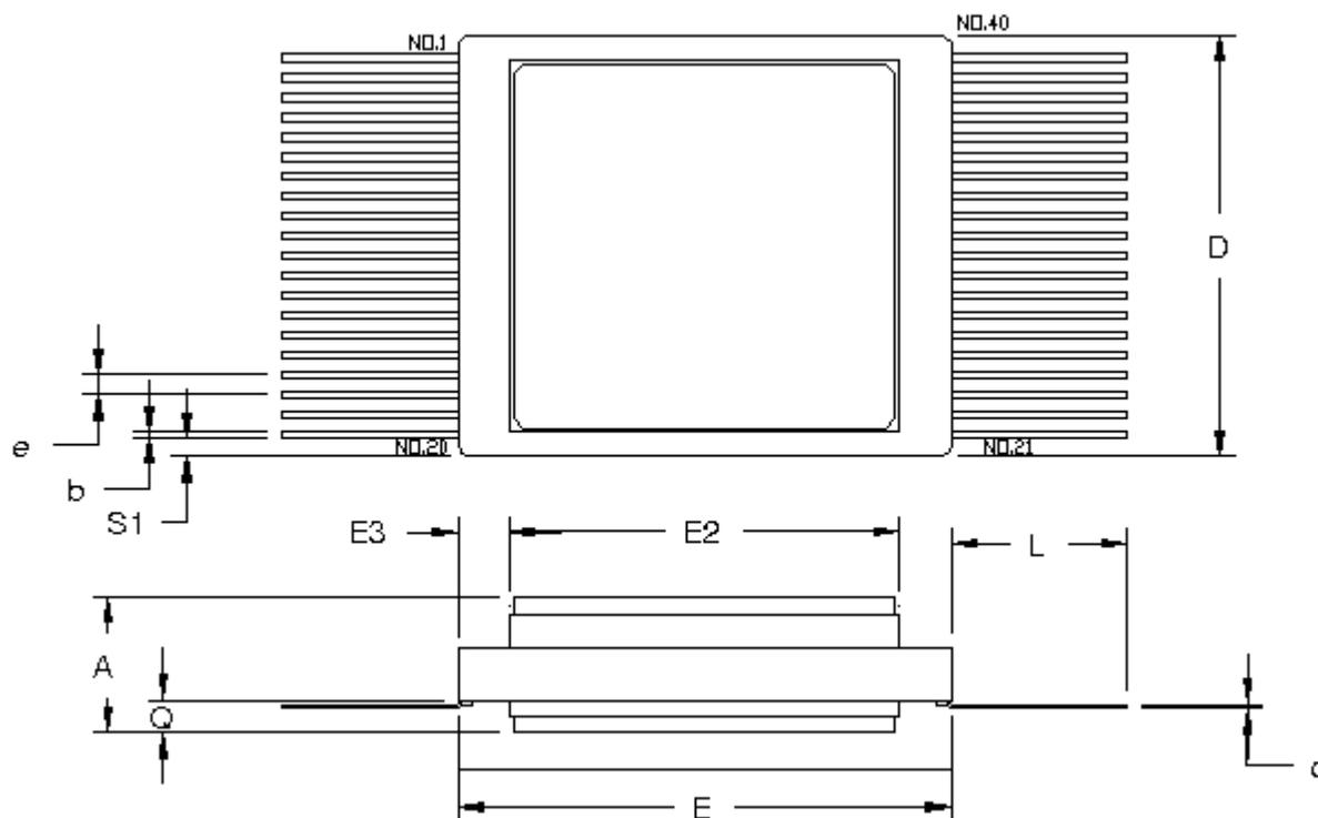
40 PIN X-RAY-PAK™ FLAT PACKAGE DIMENSIONS
