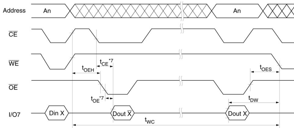
FIGURE 7. SOFTWARE DATA PROTECTION TIMING WAVEFORM(1) (IN PROTECTION MODE)
