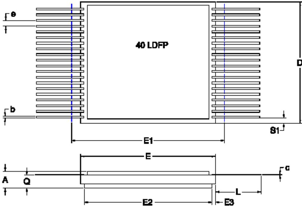
40 PIN RAD-TOLERANT FLAT PACKAGE DIMENSIONS
