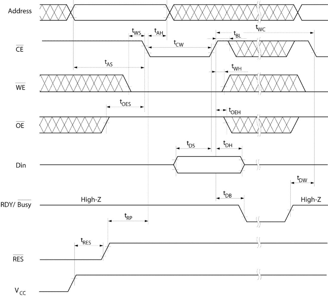
FIGURE 4. PAGE WRITE TIMING WAVEFORM(1) ( $\overline{WE}$  CONTROLLED)
