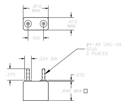
☐ RELAY HEIGHT MAY BE INCREASED .100 INCH FOR "N" SUPPRESSED COILS
