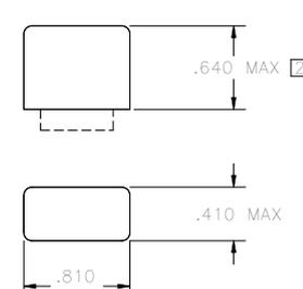
☐ RELAY HEIGHT MAY BE INCREASED .100 INCH FOR "N" SUPPRESSED COILS
