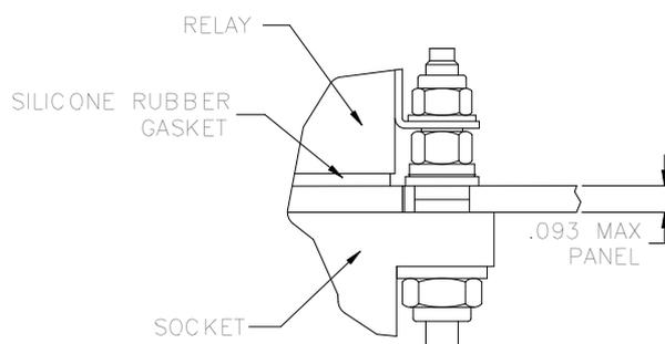
BOTTOM MOUNT-CLEARANCE HOLE FOR .164 SCREW
