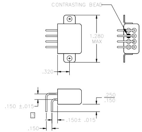
THIS END OF THE PIN WILL LIE WITHIN A CIRCULAR TOLERANCE ZONE; THE DIAMETER OF WHICH WILL BE 0.100 (8 PLACES).
