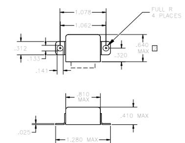
☐ RELAY HEIGHT MAY BE INCREASED .100 INCH FOR "N" SUPPRESSED COILS
