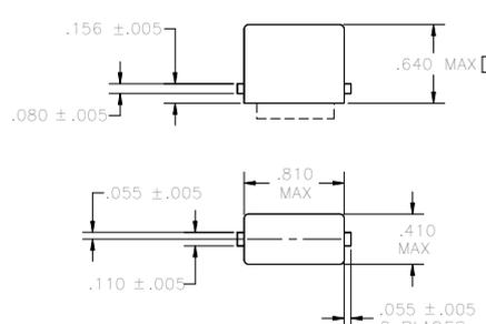
☐ RELAY HEIGHT MAY BE INCREASED .100 INCH FOR "N" SUPPRESSED COILS
