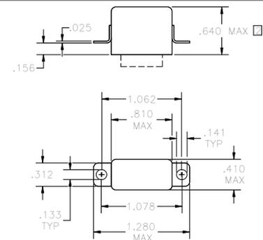
☐ RELAY HEIGHT MAY BE INCREASED .100 INCH FOR "N" SUPPRESSED COILS
