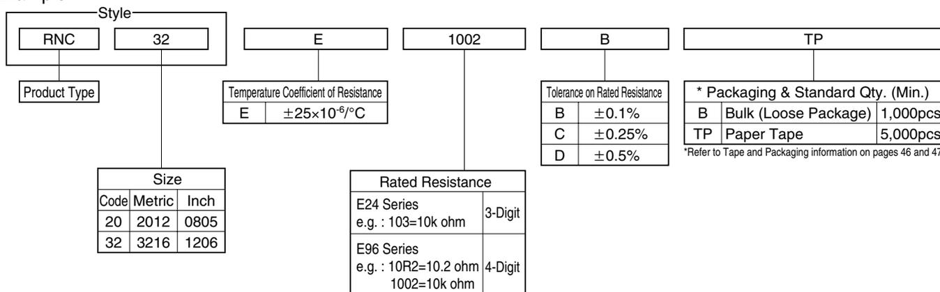
FIXED THIN FILM CHIP RESISTORS; RECTANGULAR TYPE
