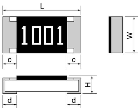
Rated resistance value is made with 3-digit (E24) or 4-digit (E96) on the over coating.
