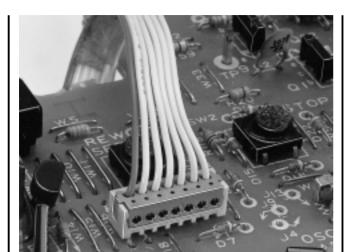
Measuring 2.0mm (.079") in pitch, only 5.0mm (.197") in mounting height, and 4.8mm (.189") in thickness, the DR connector is a compact insulation displacement connector developed to meet the needs for miniaturization of electronic equipment, including VCRs, cameras and car stereo systems.
