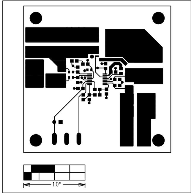
Figure 3. MAX1873 EV Kit PC Board Layout—Component Side
