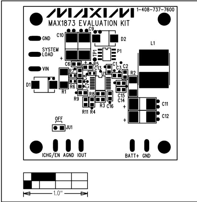
Figure 2. MAX1873 EV Kit Component Placement Guide—Component Side
