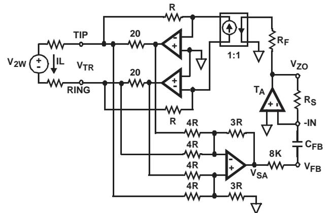
FIGURE 11. IMPEDANCE SYNTHESIS
