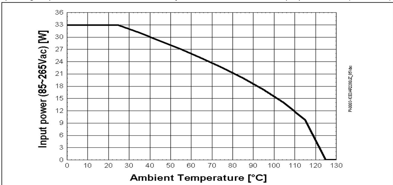
Figure 38 Input power curve  $V_{in}=85\sim 265Vac$ ;  $P_{in}=f(T_a)$
