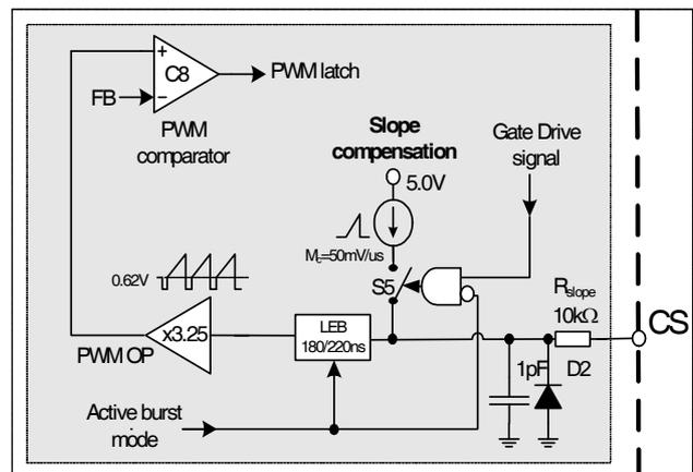
Figure 9 Slope compensation
