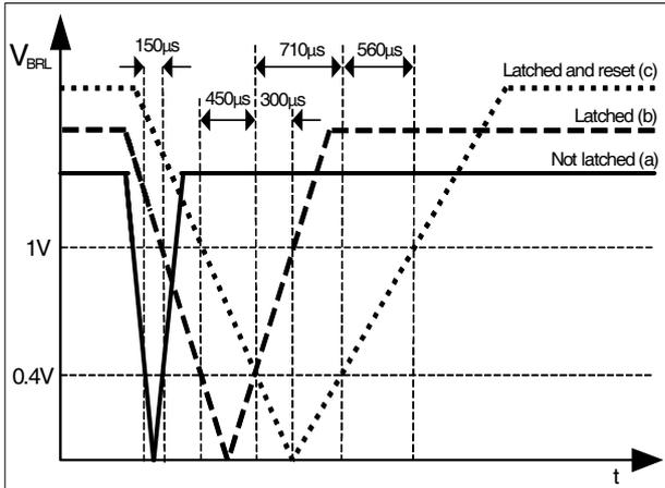
Figure 33 Latch and fast AC reset example
