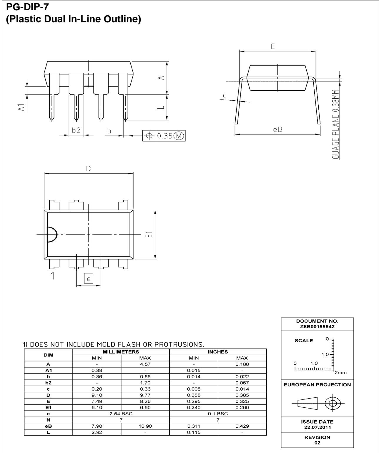
Figure 40 PG-DIP-7 (Pb-free lead plating Plastic Dual-in-Line Outline)
