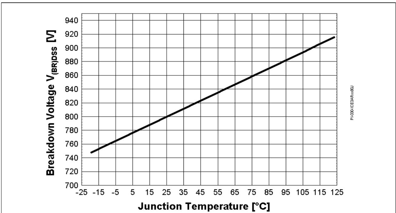
Figure 37 Drain-source breakdown voltage;  $V_{BR(DSS)}=f(T_j)$ ,  $I_D=0.25mA$
