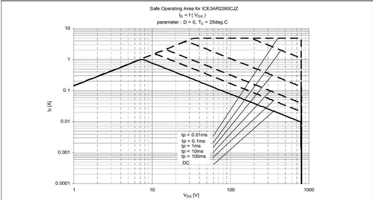
Figure 34 Safe Operating Area (SOA) curve for ICE3AR2280CJZ
