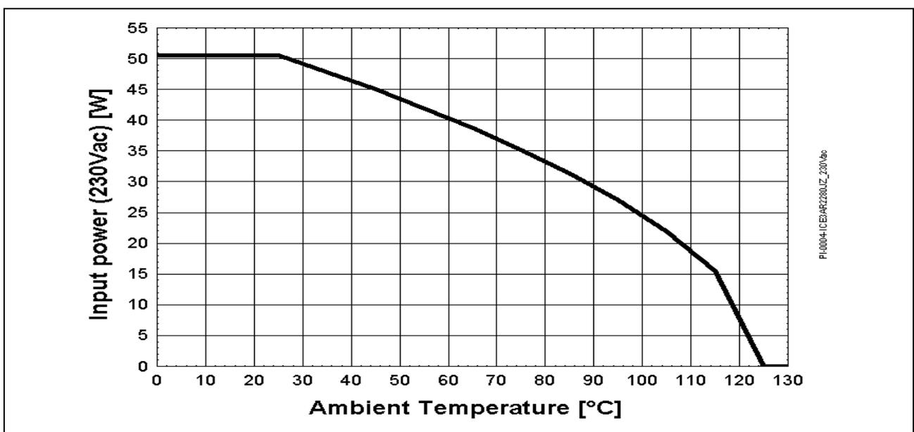
Figure 39 Input power curve  $V_{in}=230Vac\pm 15\%$ ;  $P_{in}=f(T_a)$
