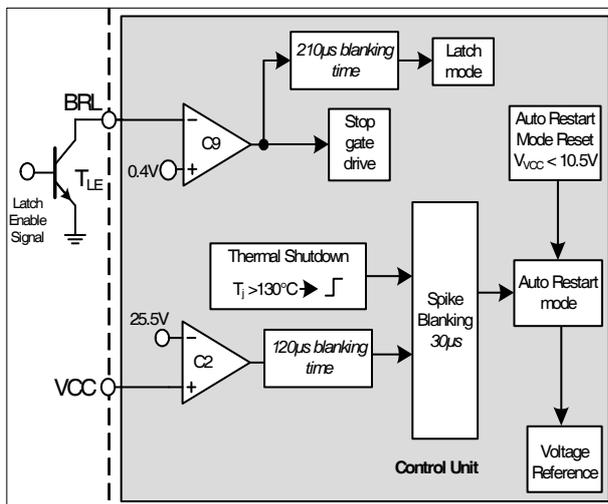
Figure 28 Vcc OVP, OTP, external protection enable
