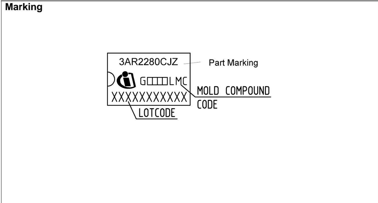
Figure 41 Marking for ICE3AR2280CJZ
