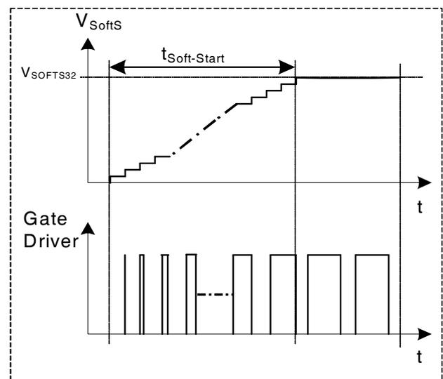
Figure 13 Gate drive signal under Soft-Start Phase
