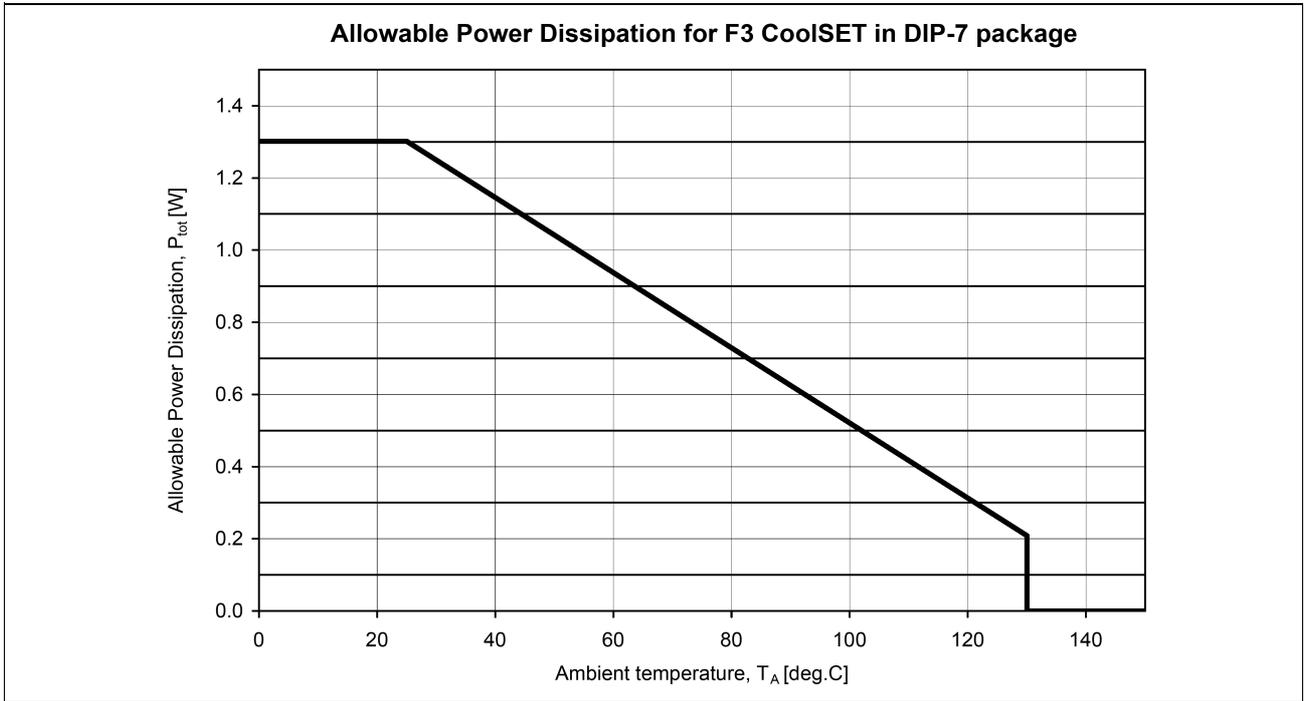
Figure 36 Power dissipation;  $P_{tot}=f(T_a)$
