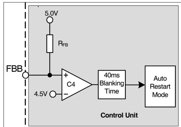
Figure 29 Over load and open loop protection
