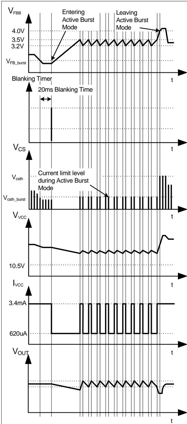
Figure 25 Signals in Active Burst Mode
