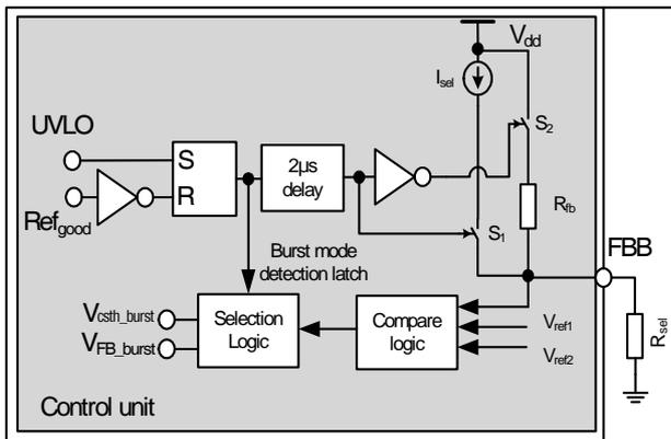
Figure 24 Burst mode detect and adjust
