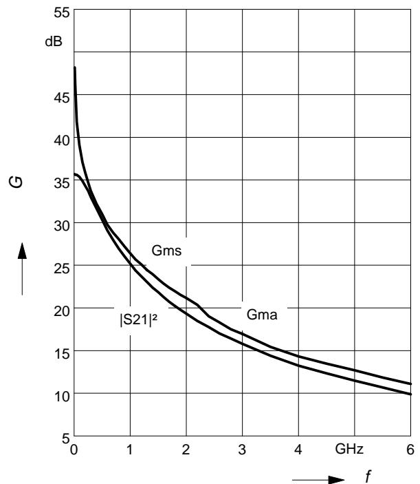
**Power gain  $G_{ma}$ ,  $G_{ms} = f(V_{CE})$**
