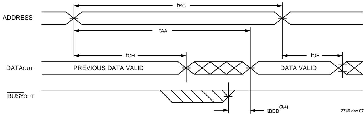
**TIMING WAVEFORM OF READ CYCLE NO. 2, EITHER SIDE<sup>(1, 3, 5)</sup>**
