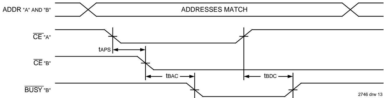
**TIMING WAVEFORM OF BUSY ARBITRATION CONTROLLED BY ADDRESSES (1)**
