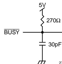
Figure 3.  $\overline{BUSY}$  AC Output Load
