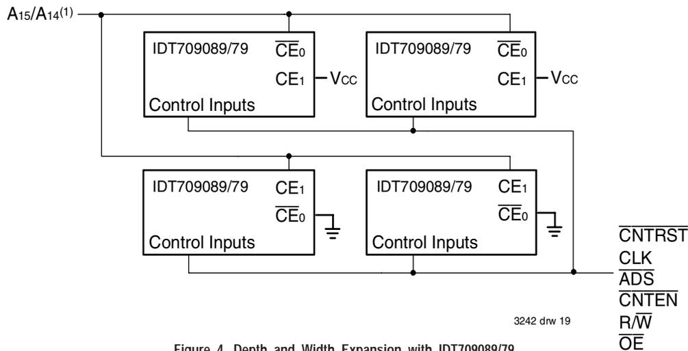
Figure 4. Depth and Width Expansion with IDT709089/79
