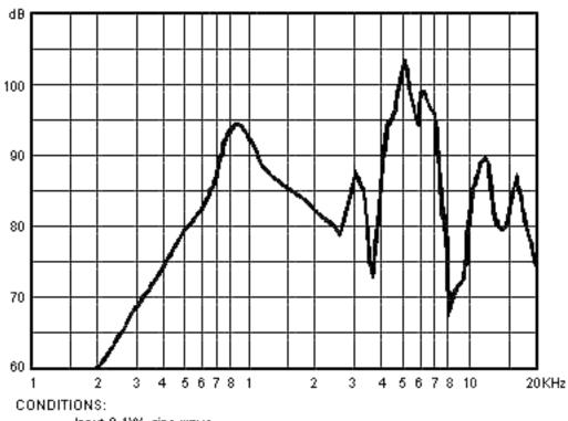
Input 0.1W sine wave Distance for measurement 10cm
