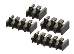
The newest product in KYOCERA AVX Interconnect family of battery connectors saves 50% in volume over the initial 9155 series compression connectors as illustrated in the photograph. These connectors are rated at a full 3 amps per contact on 2.5mm centers. Sizes range from
