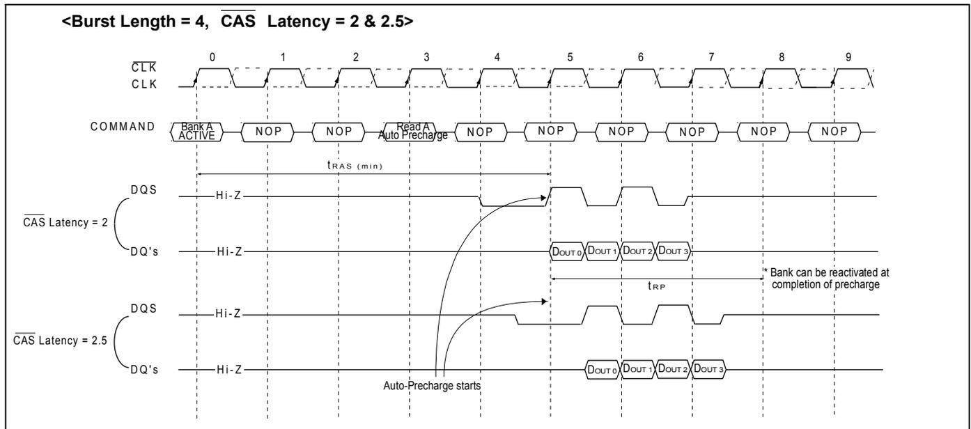
When the Read with Auto Precharge command is issued, new command can be asserted at 4, 5 and 6 respectively as follow.
