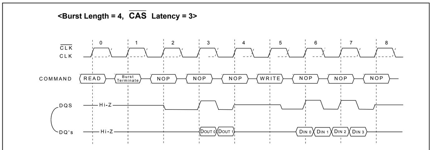
The following functionality establishes how a Write command may interrupt a Read burst.
