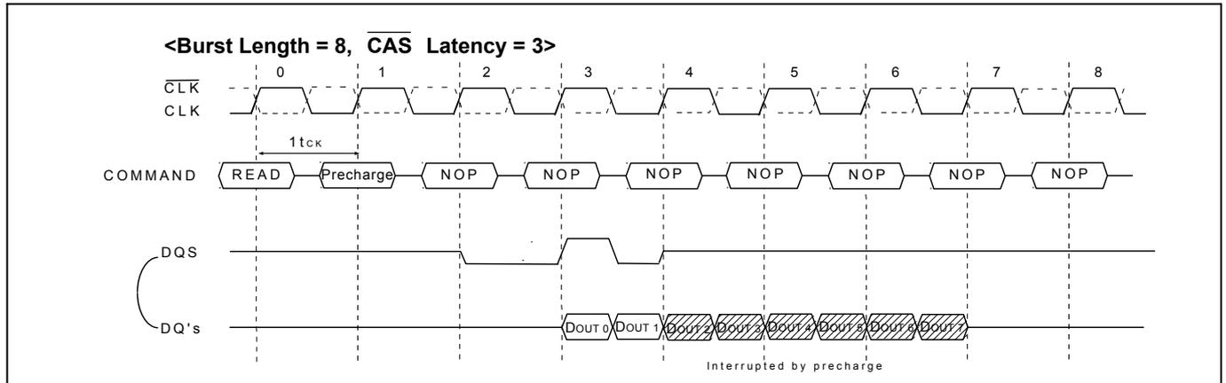
When a burst Read command is issued to a DDR SDRAM, a Precharge command may be issued to the same bank before the Read burst is complete. The following functionality determines when a Precharge command may be given during a Read burst and when a new Bank Activate command may be issued to the same bank.
