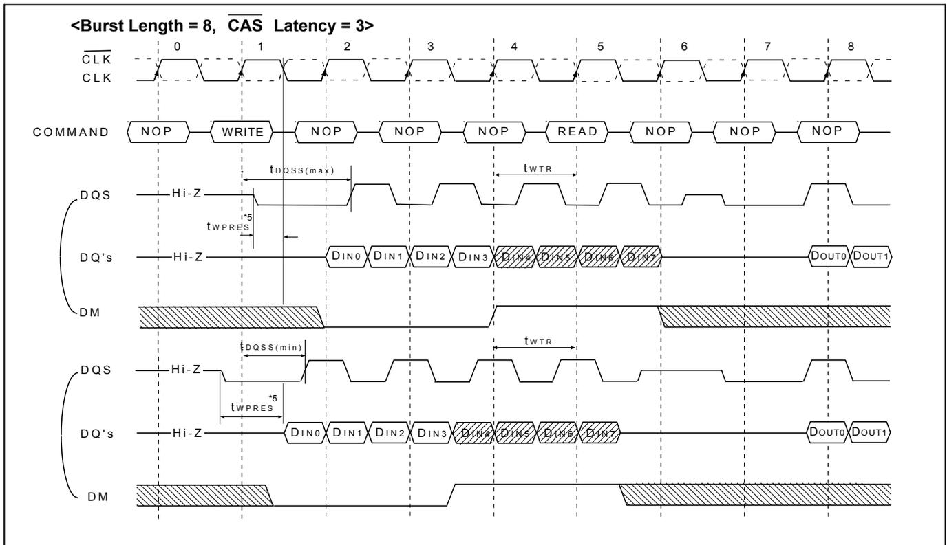
The following functionality established how a Read command may interrupt a Write burst and which input data is not written into the memory.
