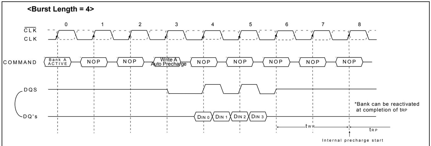
At burst read / write with auto precharge,  $\overline{\text{CAS}}$  interrupt of the same bank is illegal.
