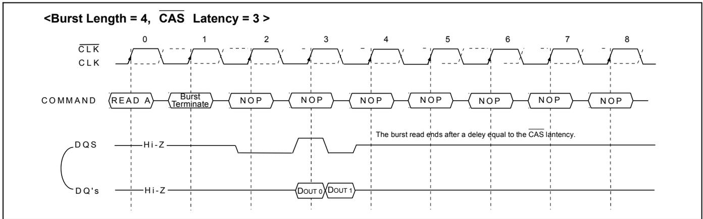
The Burst Terminate command is a mandatory feature for DDR SDRAMs. The following functionality is required.
