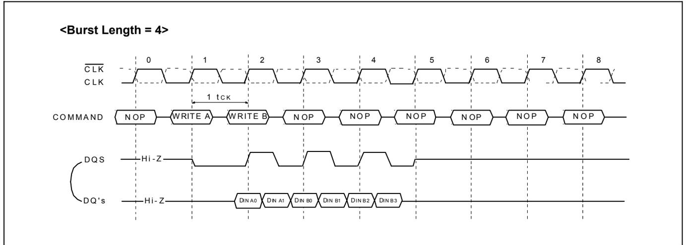
**Write Interrupted by a Read & DM**
