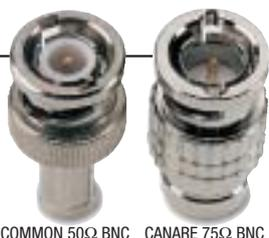
The connector on the left is a commonly used 50Ω BNC. Notice that the dielectric (white ring) is visible at the top of the outer contact.
