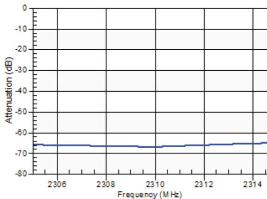
**Figure 19: Band 25 Ant-Rx Attenuation in Bluetooth/ISM Bands**
