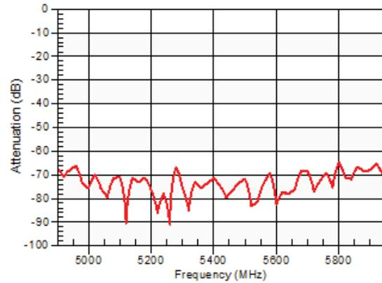
**Figure 16: Band 25 Tx-Ant Attenuation at Tx Third Harmonic**
