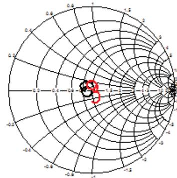
**Figure 24: . Band 25 Return Loss, Ant (black) and Rx (blue) Ports, 1930–1995 MHz**
