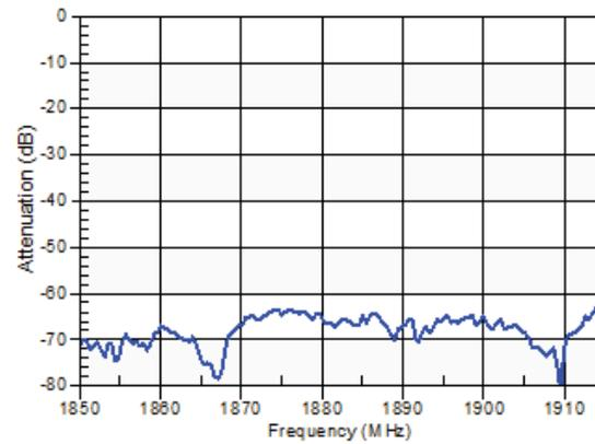
Figure 40: Band 66 Ant-Rx Attenuation in Band 30 Tx, 2305–2315 MHz
