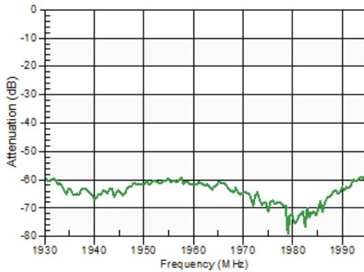
Figure 51: Cross-Band Isolation, Band 66 Tx to Band 25 Rx in Band 66 Tx, 1710–1780 MHz
