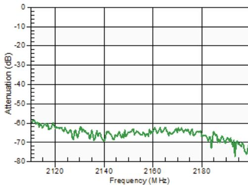
Figure 49: Cross-Band Isolation, Band 25 Tx to Band 66 Rx in Band 25 Tx, 1850–1915 MHz
