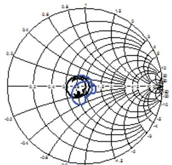
ACFM-70457045 Typical Performance at  $T_c = 25^\circ\text{C}$ , includes matching shown in Figure 1.
