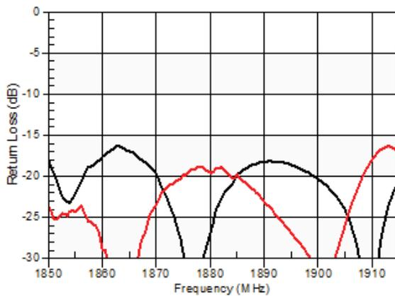
**Figure 23: Band 25 Impedance, Ant (black) and Tx (red) Ports, 1850–1915 MHz**
