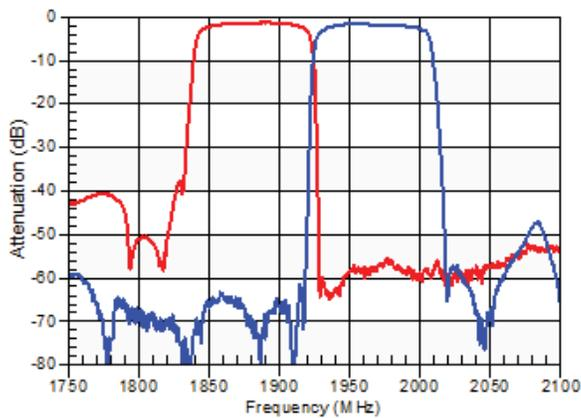
Figure 5: Band 25 Tx and Rx Port Return Loss
