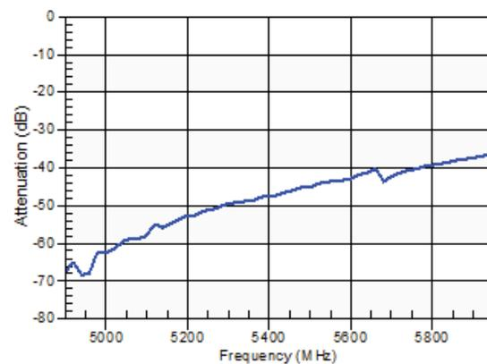
ACFM-70457045 Typical Performance at  $T_c = 25^\circ\text{C}$ , includes matching shown in Figure 1.
