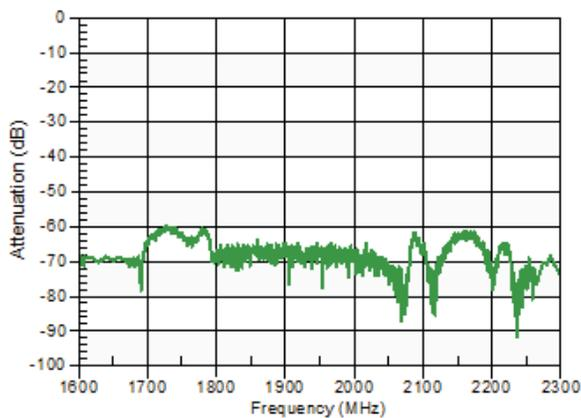
Figure 31: Band 66 Antenna Port Return Loss
