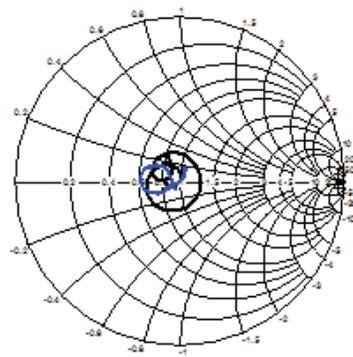
Figure 48: Cross-Band Isolation, Band 25 Tx to Band 66 Rx in Band 66 Rx, 2110–2155 MHz
