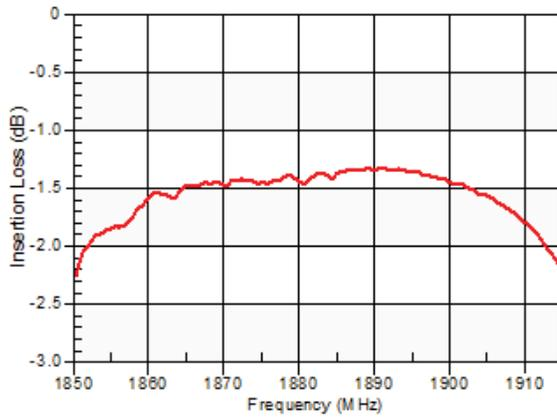
Figure 3: Band 25 Rx-Ant Insertion Loss
