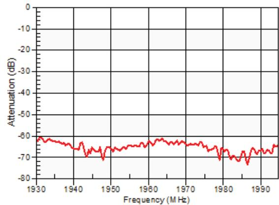
**Figure 36: Band 66 Tx-Ant and Ant-Rx Attenuation in Bluetooth Band**
