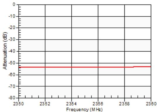
**Figure 13: Band 25 Tx-Ant Attenuation in Bluetooth/ISM Bands**
