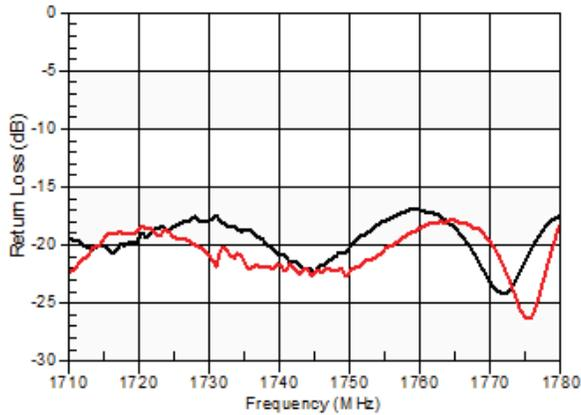
Figure 45: Band 66 Impedance, Ant (black) and Tx (red) Ports, 1710–1780 MHz
