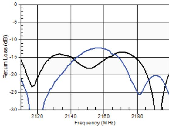
Figure 47: Band 66 Impedance, Ant (black) and Rx (blue) Ports, 2110–2200 MHz
