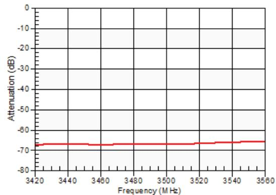
ACFM-70457045 Typical Performance at  $T_c = 25^\circ\text{C}$ , includes matching shown in [Figure 1](#).
