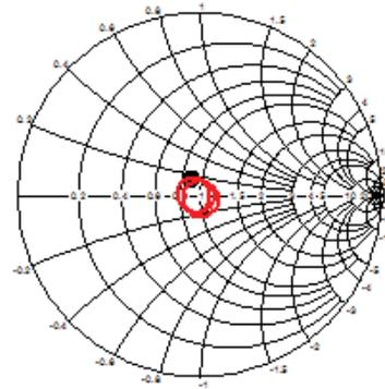
Figure 46: Band 66 Return Loss, Ant (black) and Rx (blue) Ports, 2110–2200 MHz
