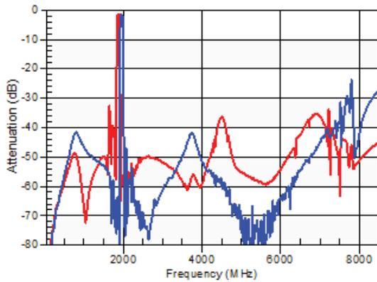
**Figure 9: Band 25 Tx-Ant and Ant-Rx Low Frequency Insertion Loss**
