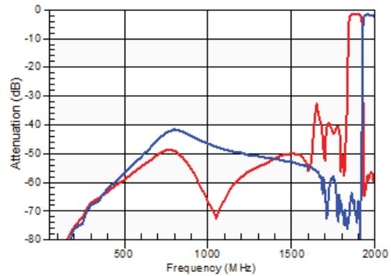
**Figure 10: Band 25 Tx-Ant Attenuation in GNSS Bands**
