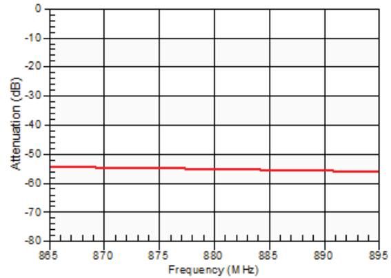
**Figure 34: Band 66 Tx-Ant Attenuation in GNSS Bands**
