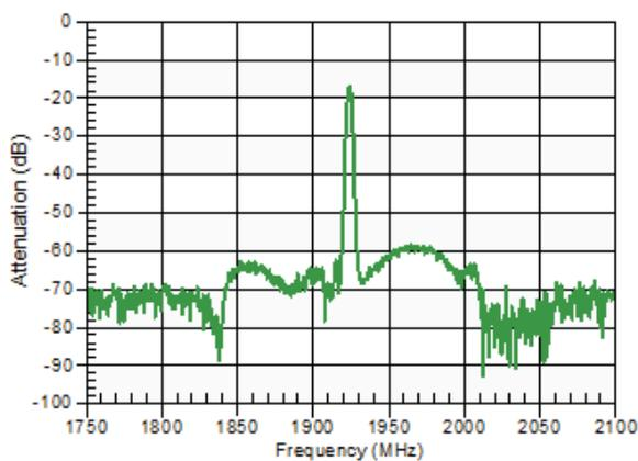
Figure 7: Band 25 Antenna Port Return Loss
