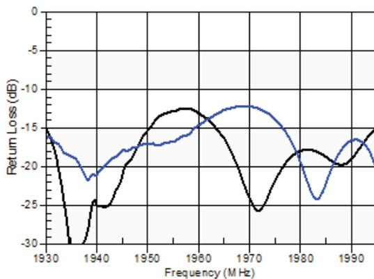
**Figure 25: Band 25 Impedance, Ant (black) and Rx (blue) Ports, 1930–1995 MHz**
