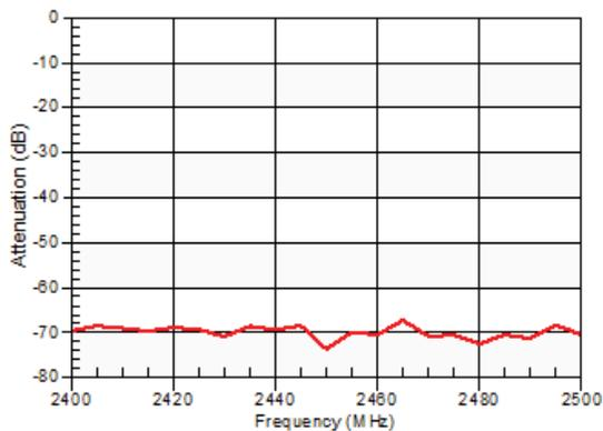
**Figure 37: Band 66 Tx-Ant Attenuation at Tx Second Harmonic**
