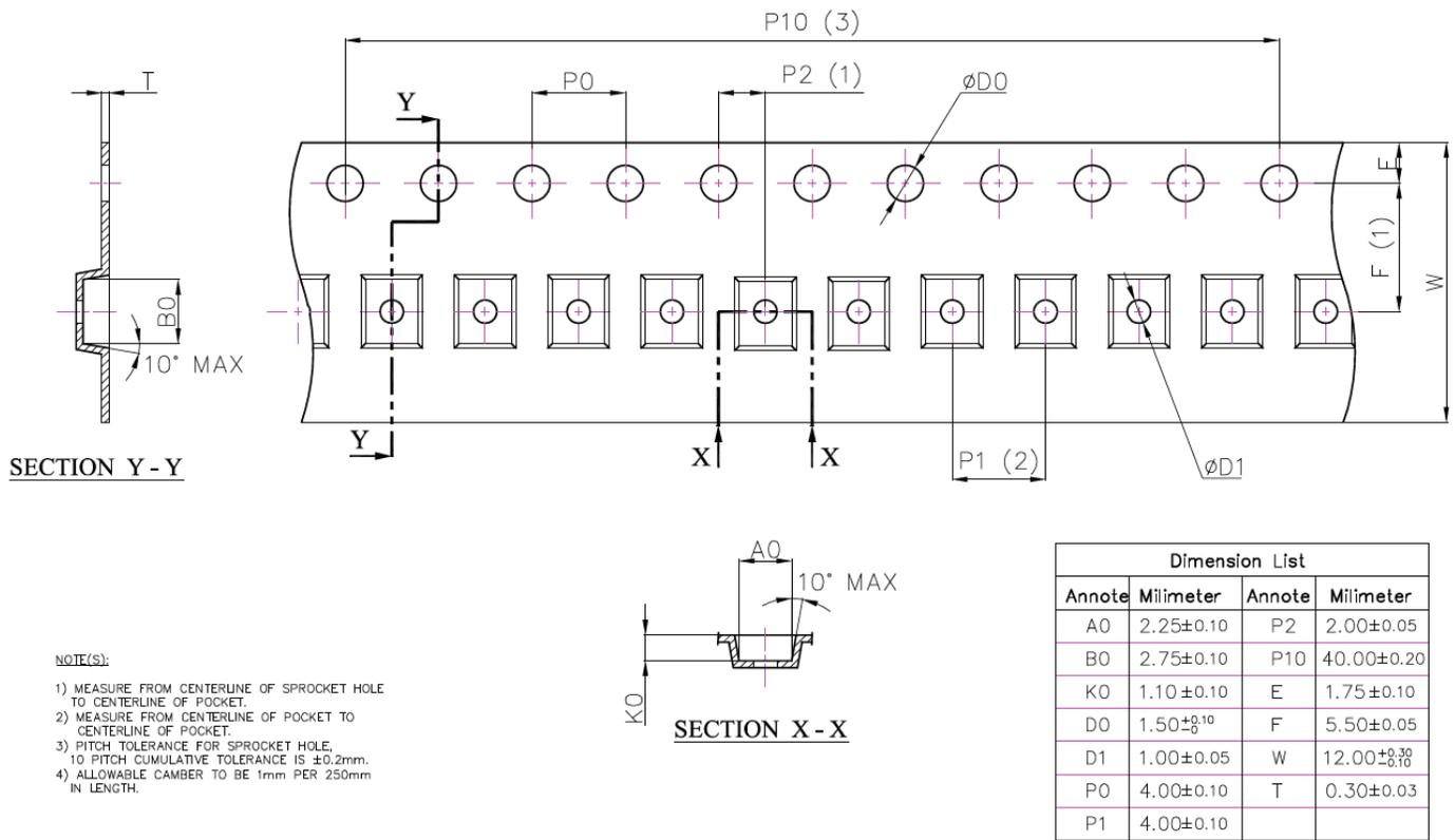
Figure 54: Orientation in Tape
