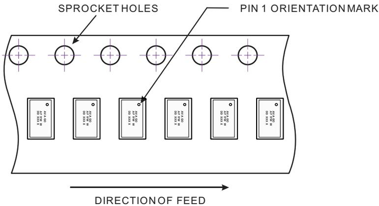
Figure 55: SMT Reel Drawing; Tape Size for ACFM-7045 is 12 mm
