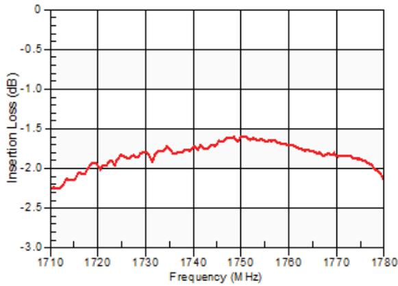
Figure 27: Band 66 Ant-Rx Insertion Loss
