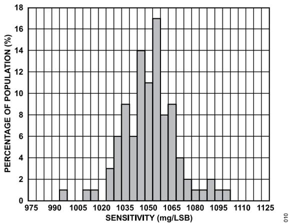
Figure 10. Z-Axis Sensitivity at 25°C, V<sub>S</sub> = 2 V, ±2 g Range
