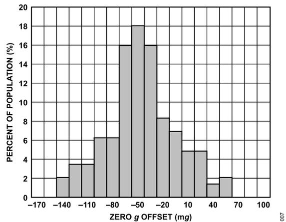
Figure 7. Z-Axis Zero g Offset at 25°C, V<sub>S</sub> = 2 V
