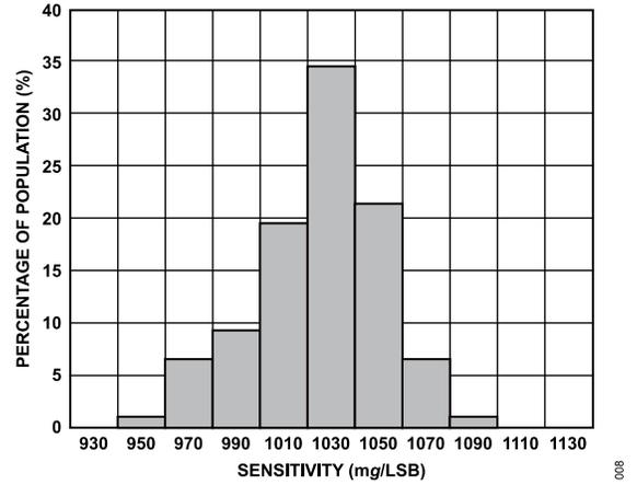
Figure 8. X-Axis Sensitivity at 25°C, V<sub>S</sub> = 2 V, ±2 g Range
