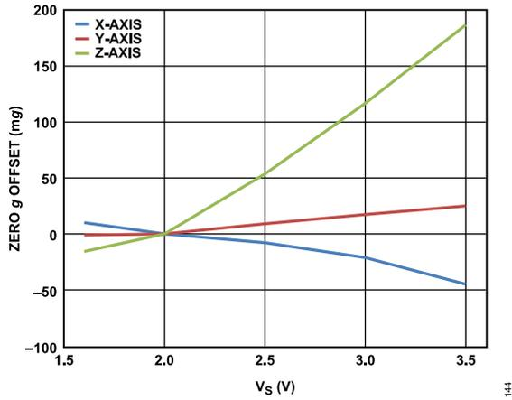
Figure 50. 0 g Offset vs. Supply Voltage
