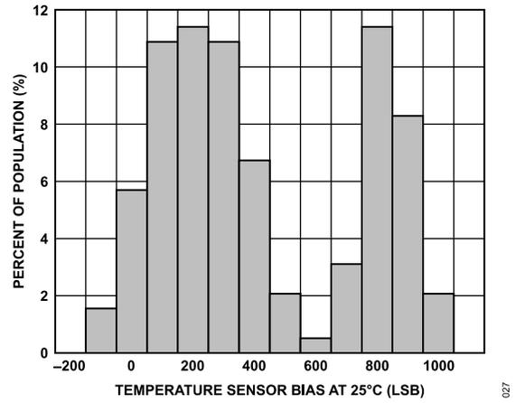
Figure 27. Temperature Sensor Response at 25°C,  $V_S = 2 V$
