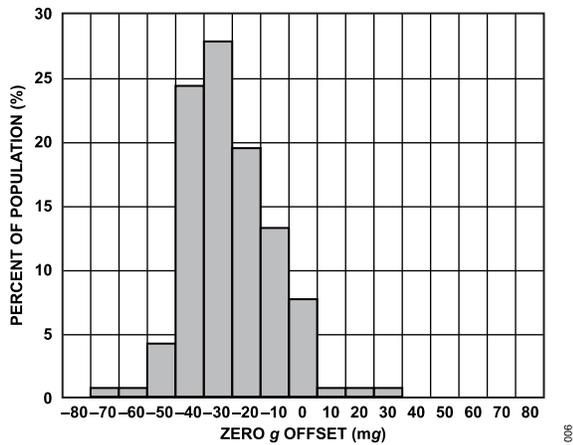
Figure 6. Y-Axis Zero g Offset at 25°C, V<sub>S</sub> = 2 V
