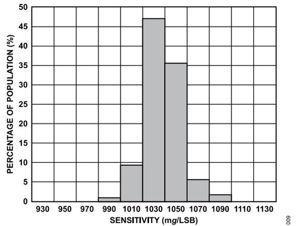
Figure 9. Y-Axis Sensitivity at 25°C, V<sub>S</sub> = 2 V, ±2 g Range
