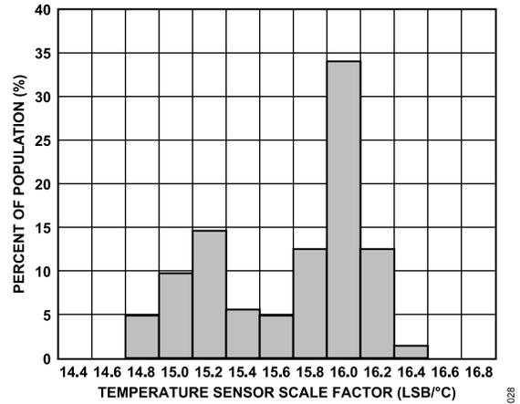
Figure 28. Temperature Sensor Scale Factor,  $V_S = 2 V$
