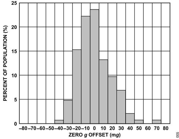
Figure 5. X-Axis Zero g Offset at 25°C, V<sub>S</sub> = 2 V
