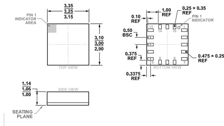
Figure 54. 16-Terminal Land Grid Array [LGA]
