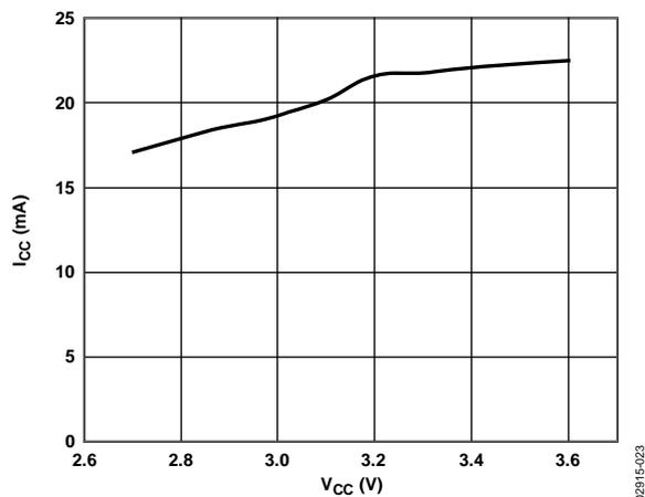
Figure 23.  $I_{CC}$  vs.  $V_{CC}$  ( $R_L = 3 k\Omega$ )
