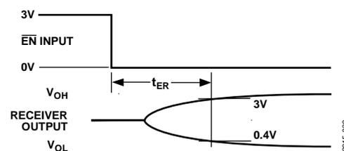
Figure 29. Receiver Enable Timing
