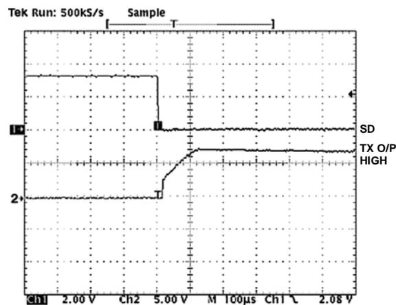
Figure 18. Transmitter Output (High) Exiting Shutdown
