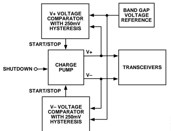
Figure 26. Block Diagram of Green Idle Circuit
