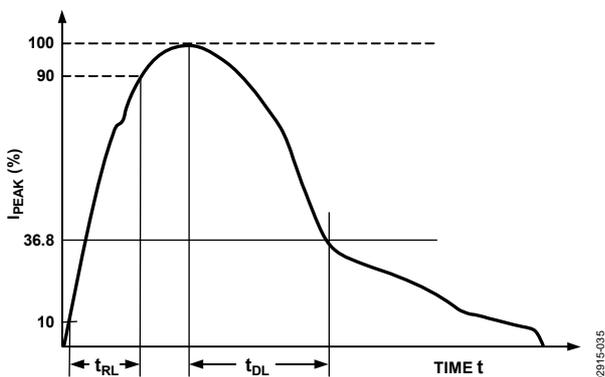
Figure 35. Human Body Model ESD Current Waveform
