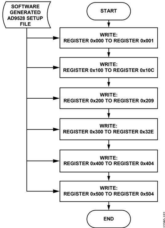
Figure 55. Subprocess, Write Registers from the Setup File
