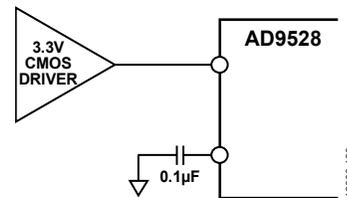
Figure 25. REFx, VCXO Input, Single-Ended Mode Receiver
