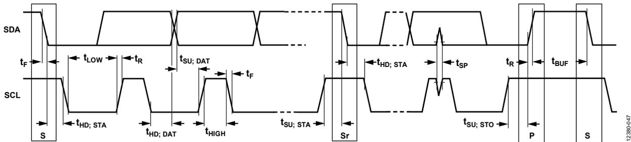
Figure 51. I<sup>2</sup>C Serial Port Timing
