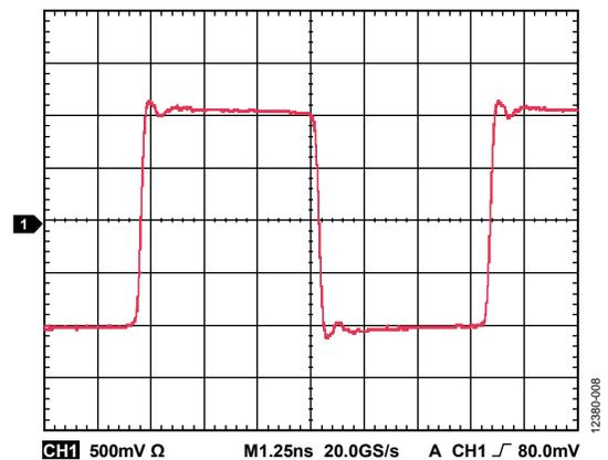
Figure 8. Output Waveform (Differential), HSTL at 122.88 MHz
