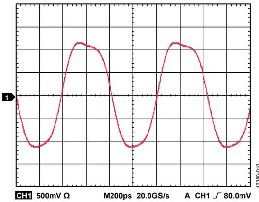
Figure 9. Output Waveform (Differential), HSTL at 1228.8 MHz
