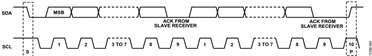
Figure 49. Data Transfer Process (Master Write Mode, 2-Byte Transfer)
