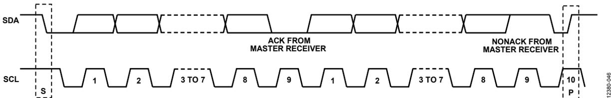
Figure 50. Data Transfer Process (Master Read Mode, 2-Byte Transfer), First ACK From Slave
