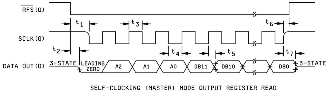
FIGURE 4. Timing waveforms - continued.
