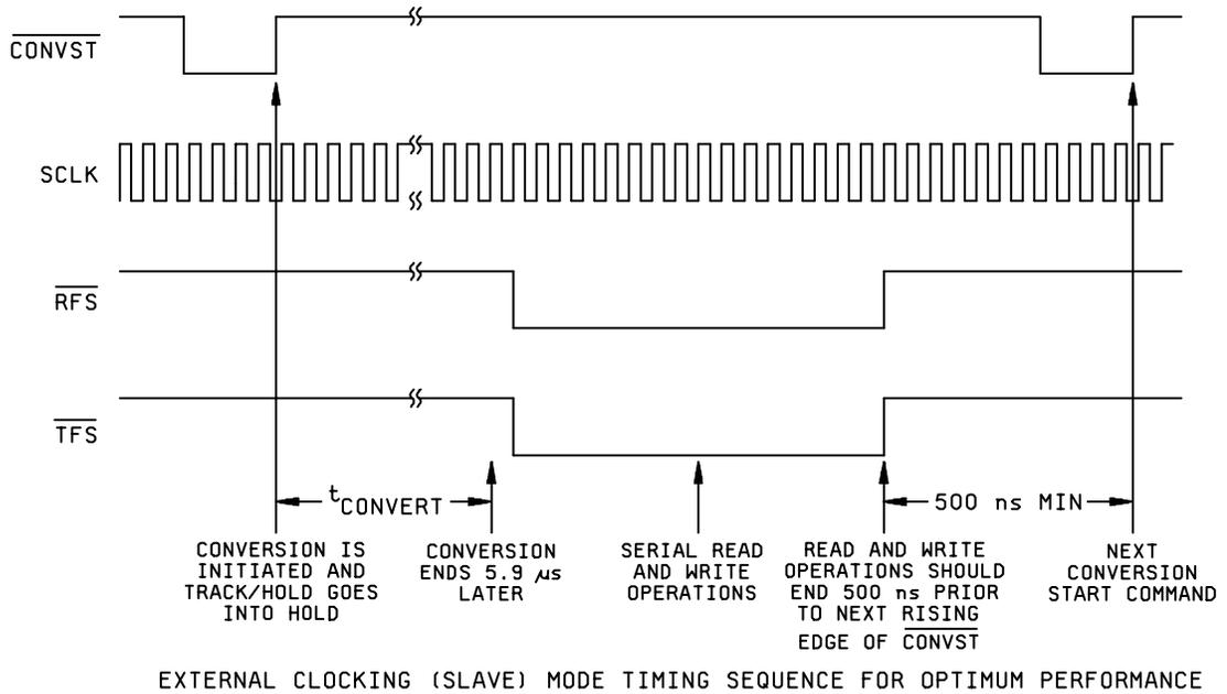
FIGURE 4. Timing waveforms.
