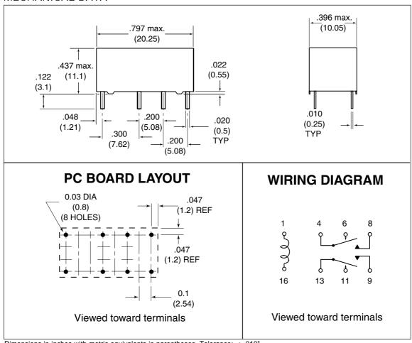
Dimensions in inches with metric equivalents in parentheses. Tolerance: ± .010"
