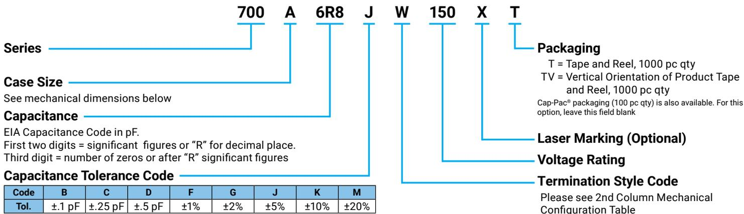
The above part number refers to a 700A Series (case size A) 6.8 pF capacitor, J tolerance (+/-5%), 150 WVDC, with W termination, (Tin/Lead, Solder Plated over Nickel Barrier), laser marking and Tape and Reel Packaging.
