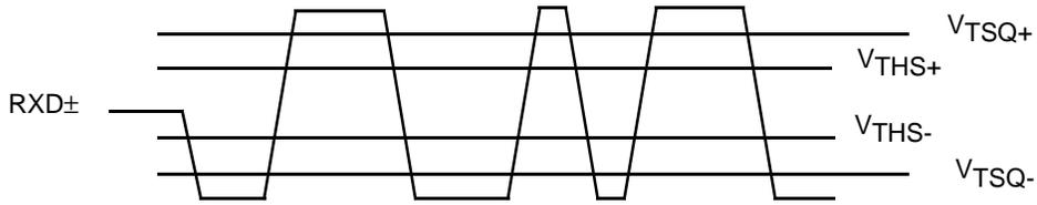
10BASE-T Receive Thresholds (LRT = 0)
