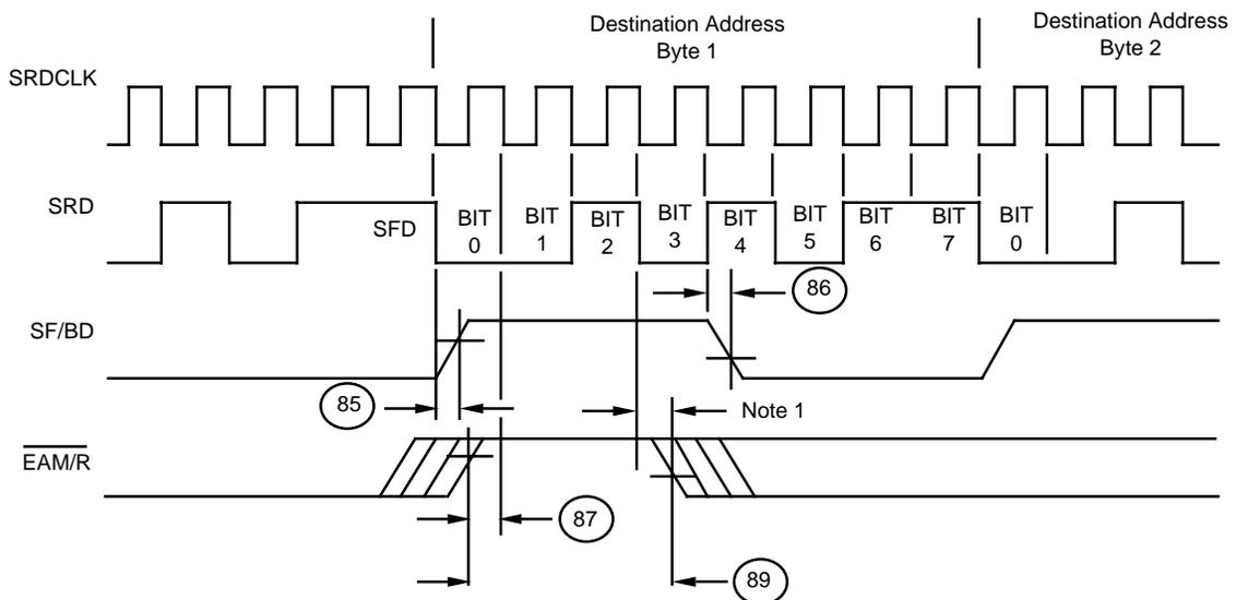
Note First assertion of  $\overline{EAM/R}$  must occur after bit 2/3 boundary of preamble.
