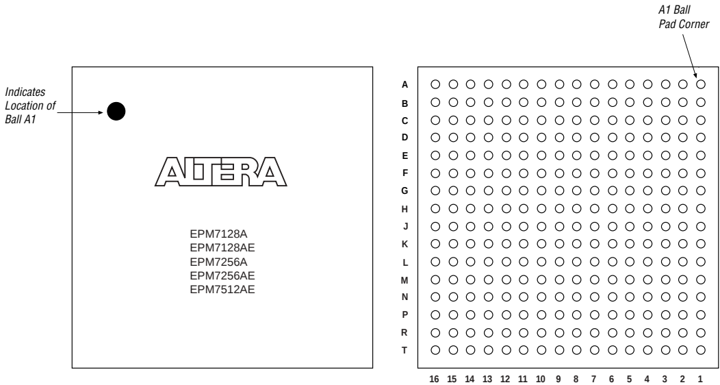
Figure 23. 256-Pin FineLine BGA Package Pin-Out Diagram
