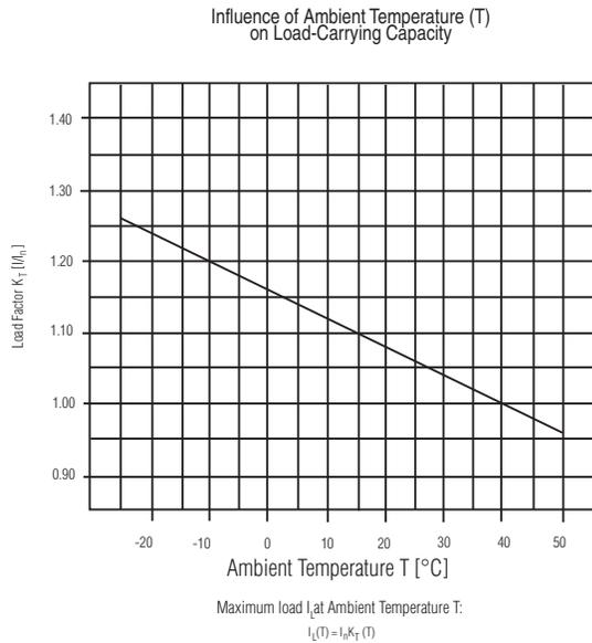
**The 1489-D circuit breaker can function over a wide temperature range (-30°...+60 °C). Operation in ambient temperatures below 0° C is based on a non condensing atmosphere (no ice). Use the graph above or contact your local Rockwell Automation sales office or Allen-Bradley distributor to determine the correction factor based upon ambient temperature.**
