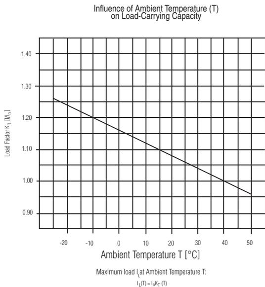
**The 1489-A circuit breaker can function over a wide temperature range (-30°...+60 °C). Operation in ambient temperatures below 0° C is based on a non condensing atmosphere (no ice). Use the graph above or contact your local Rockwell Automation sales office or Allen-Bradley distributor to determine the correction factor based upon ambient temperature.**
