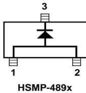
Figure 16. Internal Connections.
