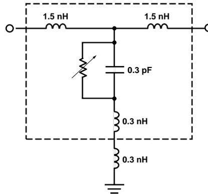
Figure 19. Equivalent Circuit.
