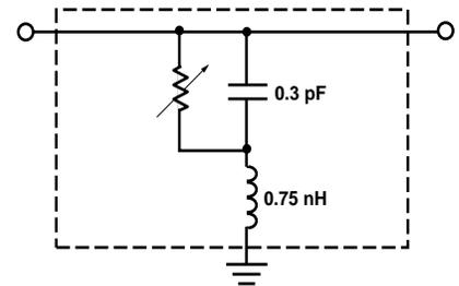
Figure 21. Equivalent Circuit.
