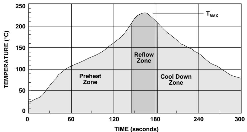
Figure 26. Surface Mount Assembly Profile.
