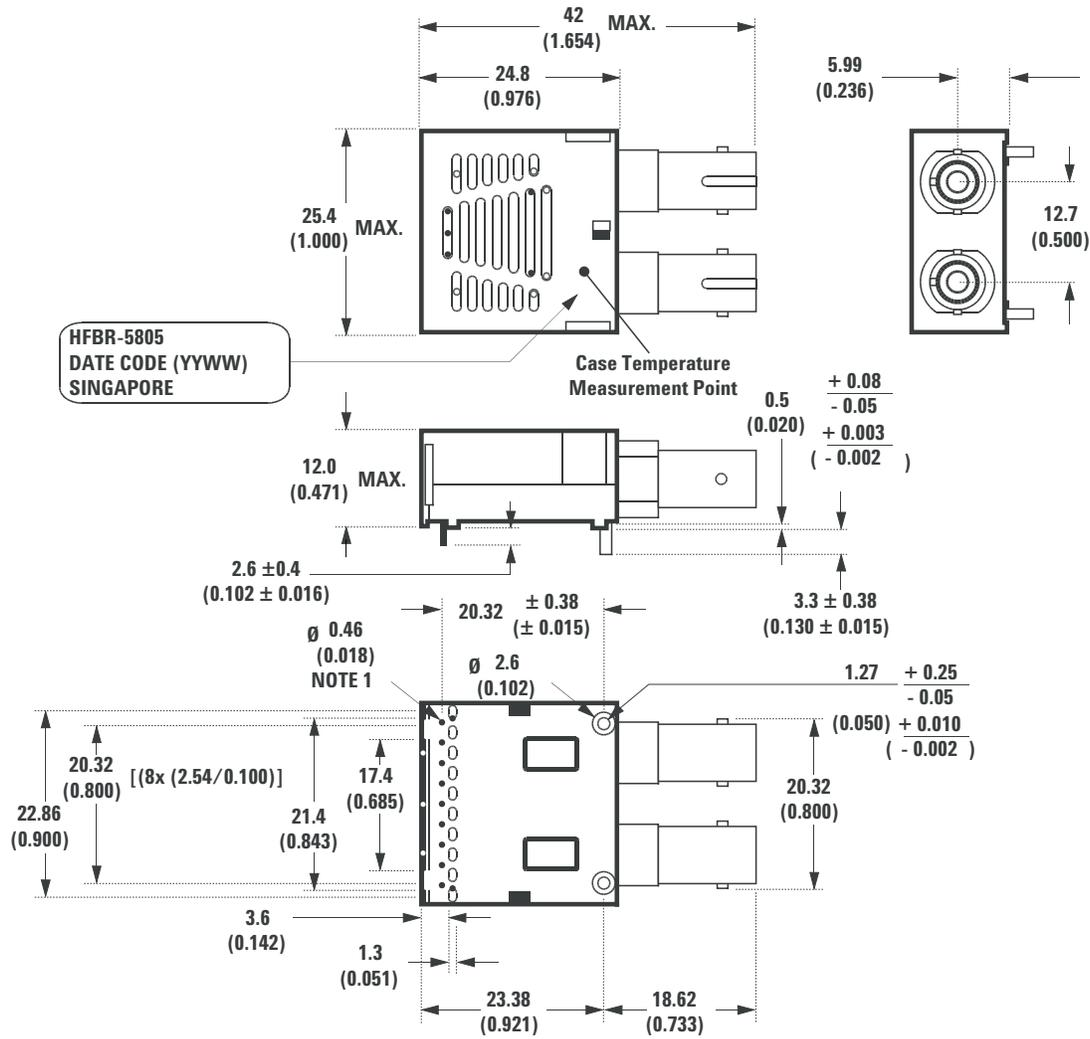
Note 1: Phosphor bronze is the base material for the posts & pins. For lead-free soldering, the solder posts have Tin Copper over Nickel plating, and the electrical pins have pure Tin over Nickel plating.
