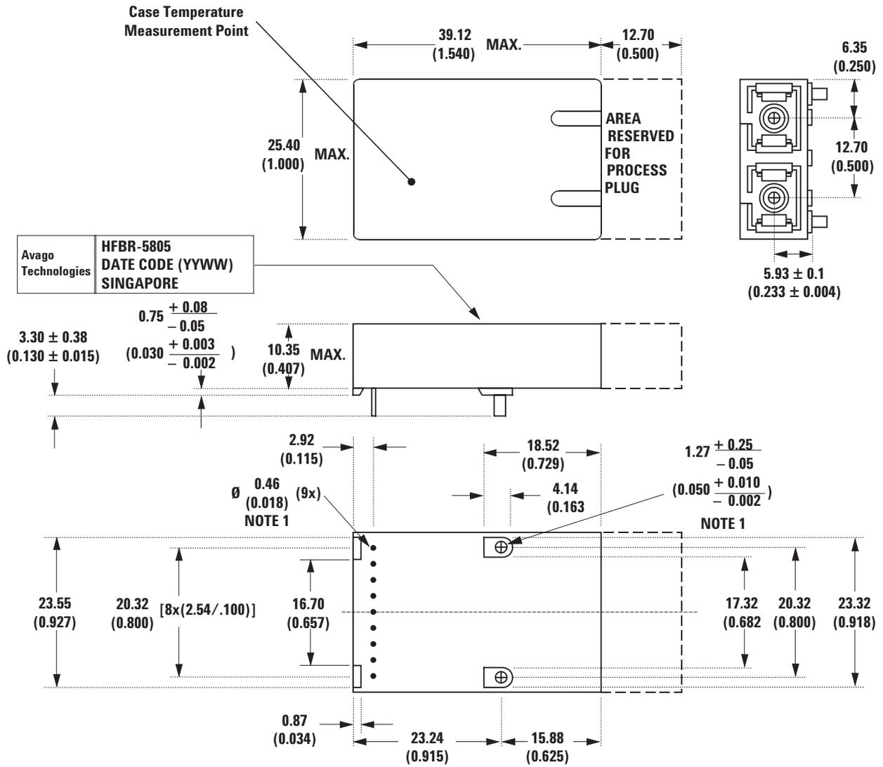
NOTE 1: THE SOLDER POSTS AND ELECTRICAL PINS ARE PHOSPHOR BRONZE WITH TIN LEAD OVER NICKEL PLATING.
