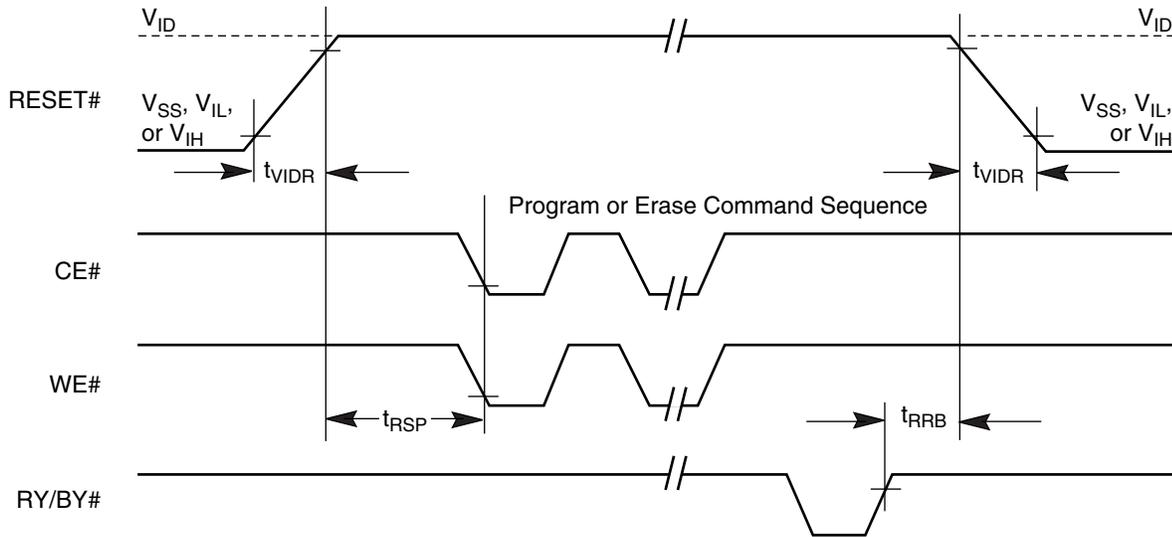
**Figure 22. Temporary Sector Group Unprotect Timing Diagram**
