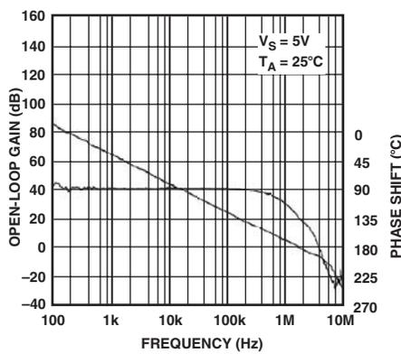
TPC 26. Open-Loop Gain and Phase vs. Frequency,  $V_S = 5V$
