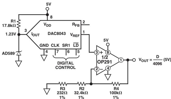
Figure 9. 5 V Only, 12-Bit DAC Swings Rail-to-Rail
