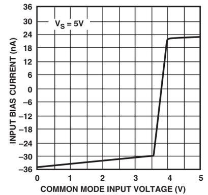
TPC 24. Input Bias Current vs. Common-Mode Input Voltage,  $V_S = 5V$
