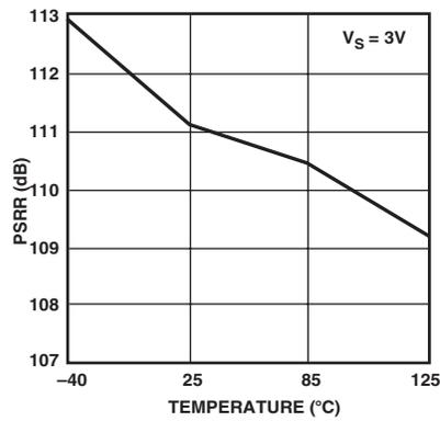
TPC 14. PSRR vs. Temperature,  $V_S = 3\text{ V}$
