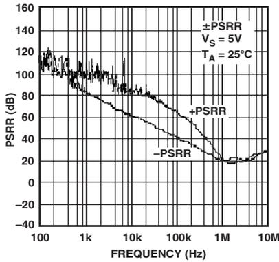
TPC 31. PSRR vs. Frequency,  $V_S = 5\text{ V}$
