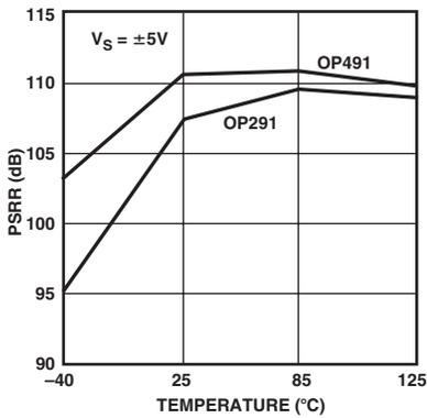
TPC 49. OP291/OP491 PSRR vs. Temperature,  $V_S = \pm 5\text{ V}$
