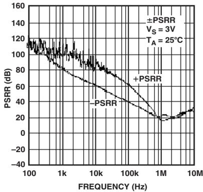
TPC 13. PSRR vs. Frequency,  $V_S = 3\text{ V}$
