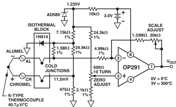
Figure 11. A 3 V, Cold-Junction Compensated Thermocouple Amplifier
