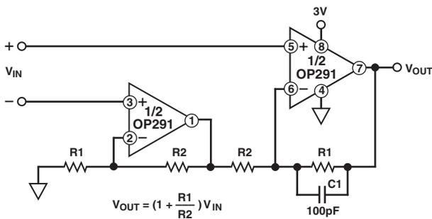
Figure 6. Single 3 V Supply Instrumentation Amplifier
