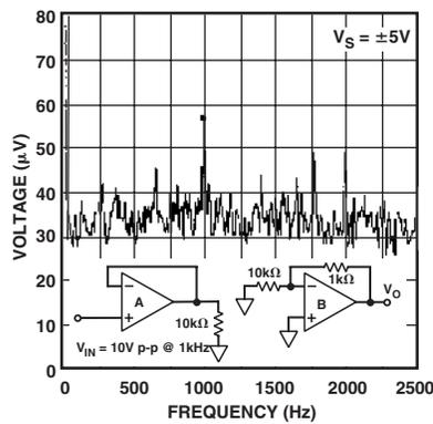
TPC 35. Channel Separation,  $V_S = \pm 5\text{ V}$
