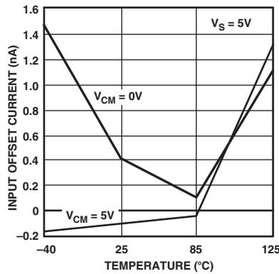
TPC 23. Input Offset Current vs. Temperature,  $V_S = 5V$
